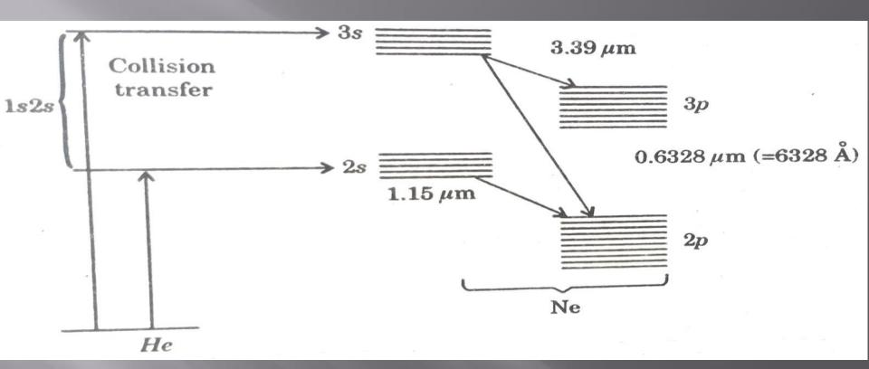
□ Excited He atoms collide with unexcited neon atoms and resonant energy transfer takes place so that neon atoms get excited to a specific energy level.
